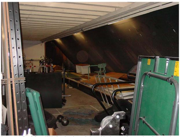
Room 114, Reed Gym, ISU, showing the angled metal backstop and covered sand trap on the right side of the photo. Photo taken on 5/18/2011. Lead wipe samples were highest on the floor in front of the trap (center of the photo) and on the overhead light fixture diffuser plates.
